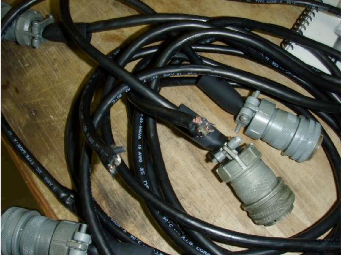
**Image A2: Damaged battery cables from Minna Bluff AWS**
