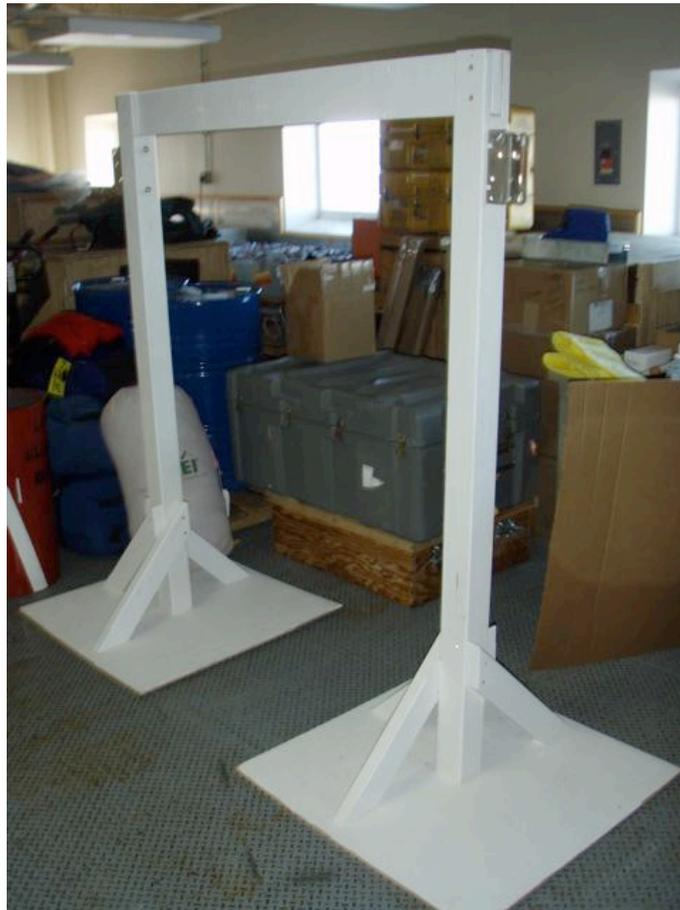
**Figure 2. Mounting platform for radiation shield/temperature sensor testing.**
