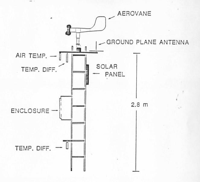
Figure 3. Layout of the AWS unit used in Antarctica. Nine gel cell batteries of 40 ampere hour capacity each are used in the cold regions of Antarctica such as South Pole and six batteries are used in the warmer regions such as the Ross Ice Shelf.
